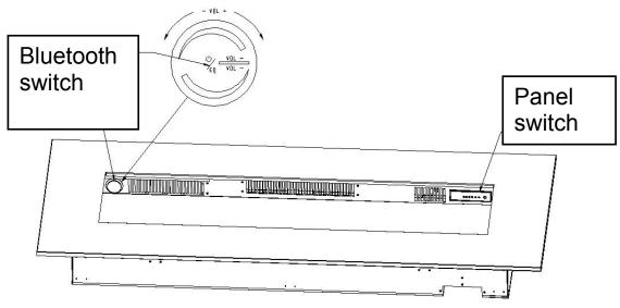
3.1 Long press the speaker boot and connect the speaker with a Bluetooth device
