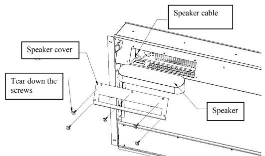
Tear down the screws on the speaker cover, Take out the speaker, Plug out the speaker cable, and cover the speaker
